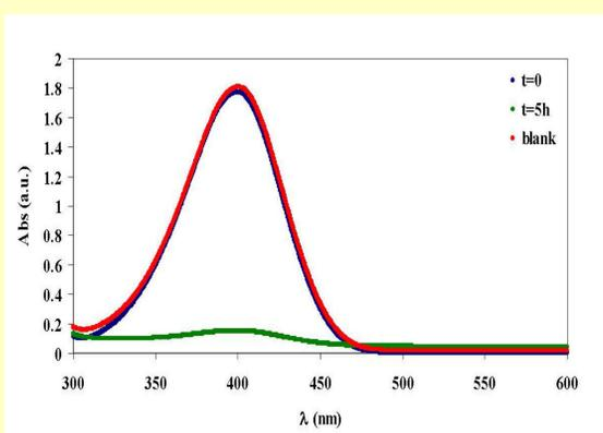
UV-Vis spectra of p-nitrophenol (PN) aqueous solutions. *Blue*: [PN]=1x10<sup>-4</sup> M before the addition of cellulose. *Green*: 5 hours after the addition of modified cellulose I. *Red*: 5 hours after the addition of non-modified cellulose D.
