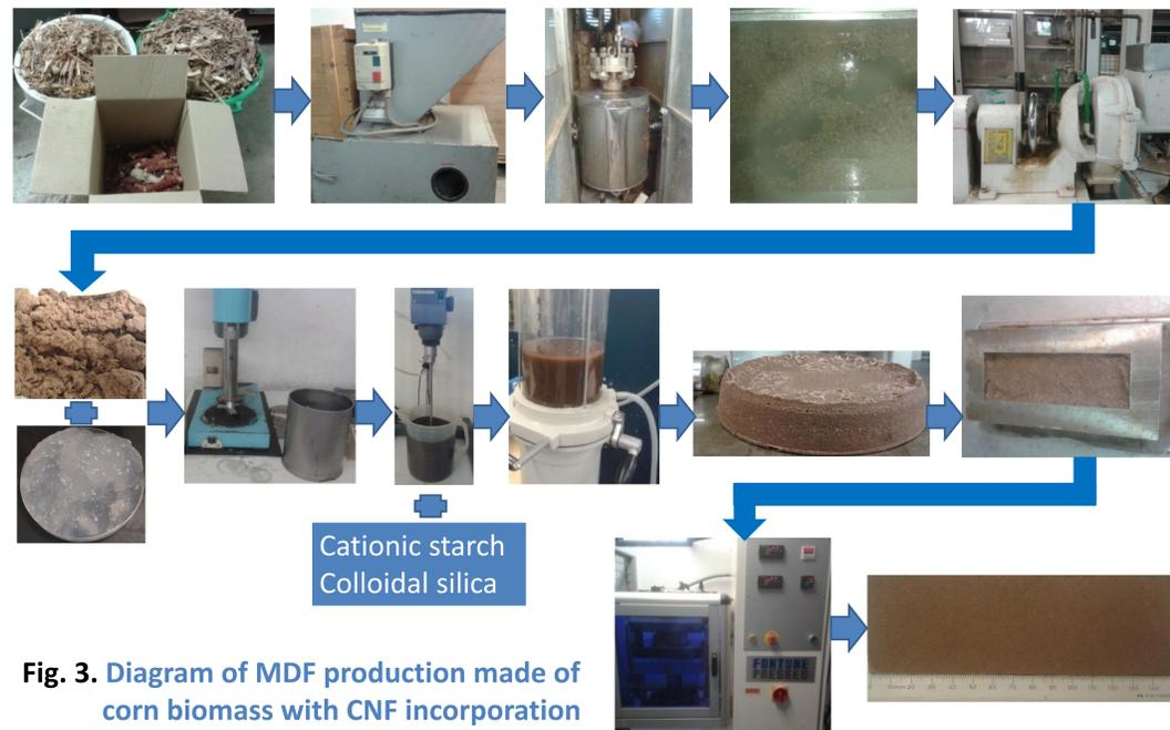
Fig. 3. Diagram of MDF production made of corn biomass with CNF incorporation
