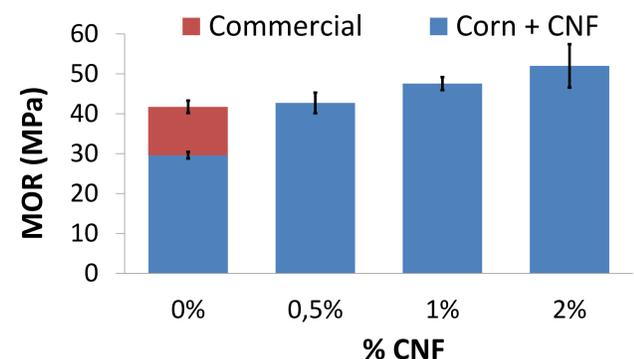
Fig. 4. Modulus of Rupture (MOR) of MDF made of corn biomass with %CNF and commercial MDF
