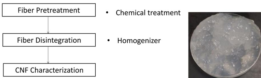
Fig. 2. Main processes involved in producing CNF from Eucalyptus pulp and 5 mmol CNF
